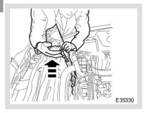
Remove the timing cover, step 3.
