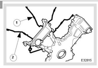
Remove and discard the inner and outer seals from the timing cover.
