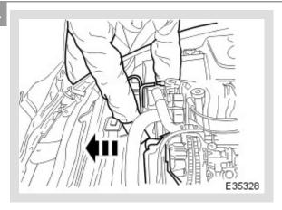
Remove the timing cover, step 1.
