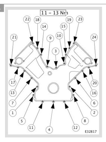
Fit and tighten the securing bolts in the correct order. Tighten to 11-13 Nm.
