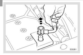
Disconnect the battery ground cable.
