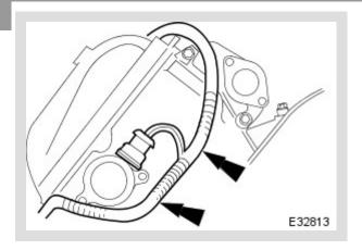
Reposition and secure the engine harness clips to the timing cover.
