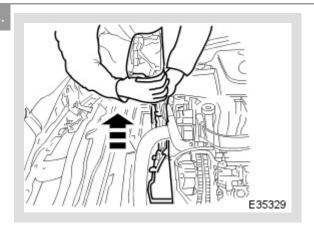
Remove the timing cover, step 2.
