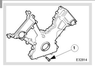
Remove the timing cover securing bolts.
