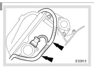
Disconnect the engine harness retaining clips from the timing cover.
