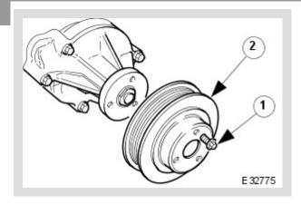
Remove the pulley from the water pump.
