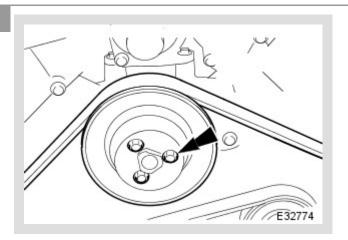
Slacken the three screws which secure the water pump pulley.
