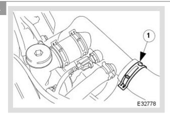
Disconnect the top hose from the coolant outlet pipe.
