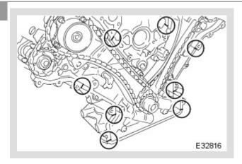
Apply sealant to the eight joints on the engine face.
