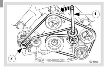
Remove the drive belt from the generator and accessory drive.
