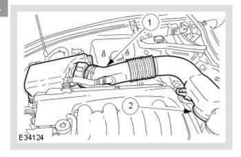
Remove the intake tube / air flow meter / air cleaner cover assembly.
