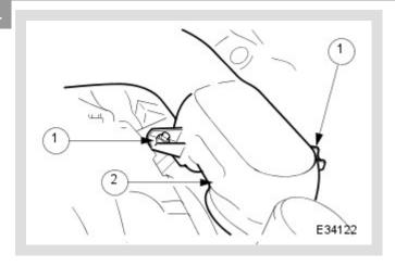
Disconnect the intake tube from the throttle body.
