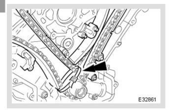
Fit a Tie-Strap through the links of the primary chain, just above the crankshaft sprocket, to retain the chain to the sprocket.
