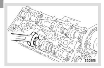
Rotate the inlet camshaft (and the exhaust camshaft), using a spanner on the flats, to provide sufficient slack in the chain to remove the chain guide.
