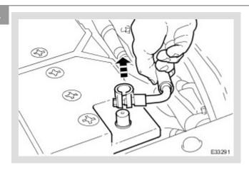
Disconnect the battery ground cable.
