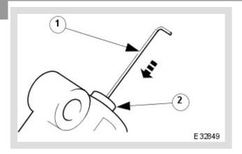
Push the tensioner piston into the body to provide clearance for fitting.
