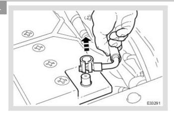
Disconnect the battery ground cable.
