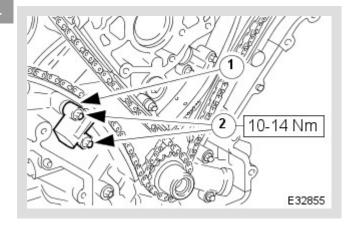
Fit the tensioner to the cylinder block.
