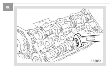
Rotate the inlet camshaft (and the exhaust camshaft), using a spanner on the flats, to provide sufficient slack in the chain to remove the chain tensioner blade.
