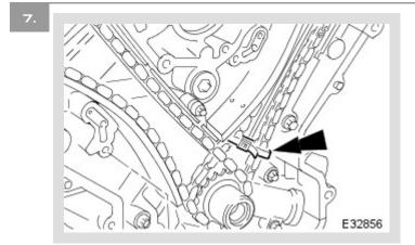
Fit a Tie-Strap through the links of the primary chain, just above the crankshaft sprocket, to retain the chain to the sprocket.
