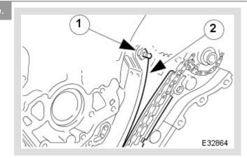
Remove the chain tensioner blade.
