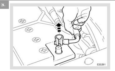
Disconnect the battery ground cable.
