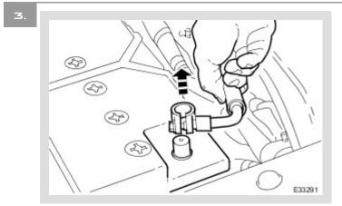
Disconnect the battery ground cable.
