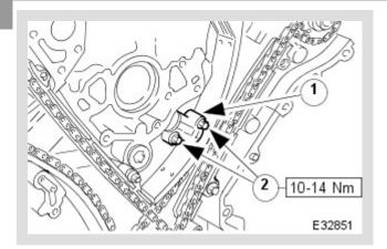
Fit the tensioner to the cylinder block.
