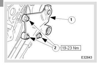
Fit the bush carrier to the cylinder block.
