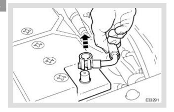
Disconnect the battery ground cable.
