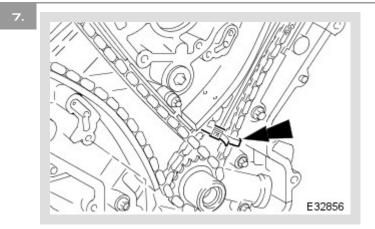
Fit a Tie-Strap through the links of the primary chain, just above the crankshaft sprocket, to retain the chain to the sprocket.
