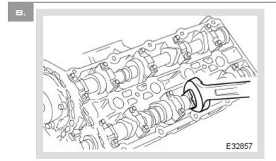
Rotate the inlet camshaft (and the exhaust camshaft), using a spanner on the flats, to provide sufficient slack in the chain to remove the chain guide.
