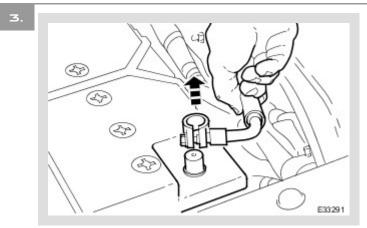
Disconnect the battery ground cable.
